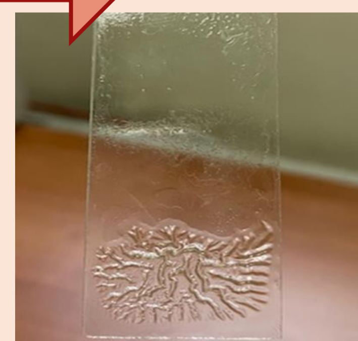
Figure 9 UV cured formulation of 0.1% w/w of [E]-1-4NMAPE-one, %99 TPGDA, %1 NMDEA and irradiation time is 135 seconds.
